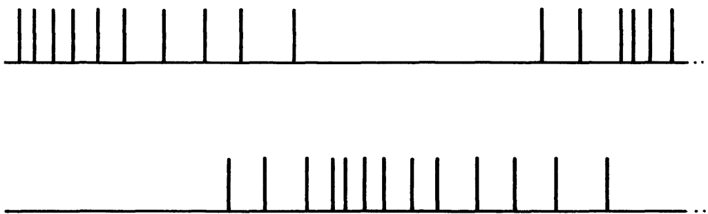
Figure 10. Multivibrator effect with overlapping switchovers.
